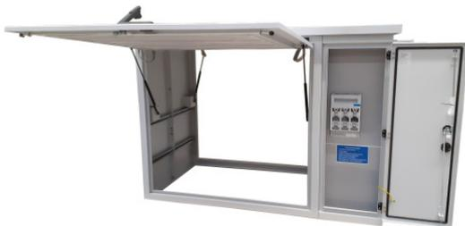
BxHxT: 1700(1300+400)x1300x1000mm, aus AlMg3, kunststoffbeschichtet in RAL7035, IP43, Trafoabmessungen max: BxHxT: 900x900x750mm
